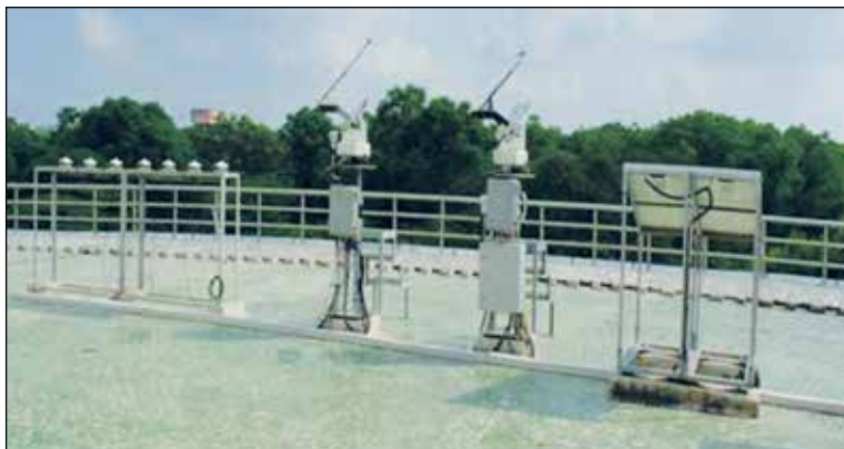
Fig. 10.7: Calibration of Radiometers at NISE
