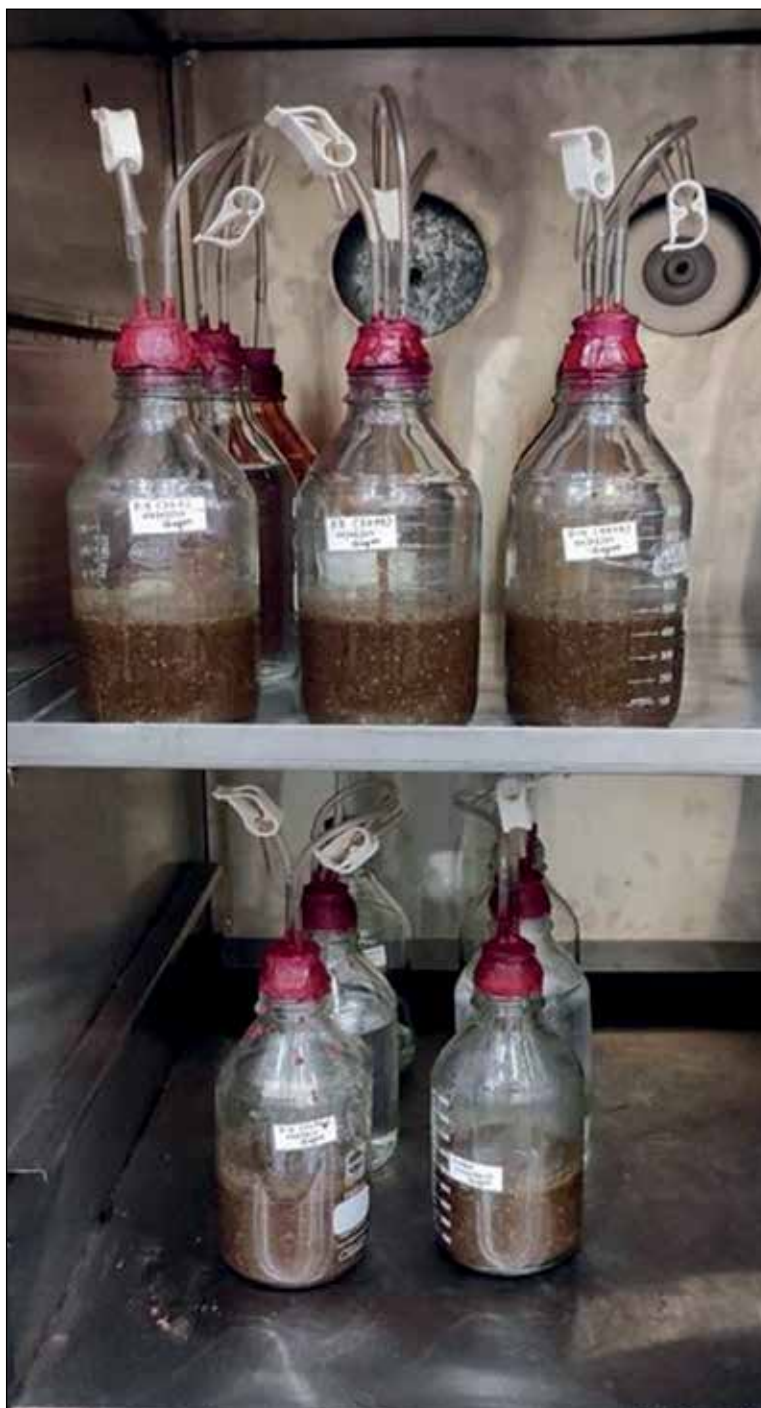
Fig. 10.16: Laboratory-scale plants for biogas production from water hyacinth having different thermophilic inoculums
