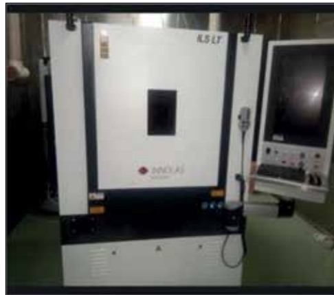
Fig. 7.13: Laser system installed at BHEL ASSCP (capable of laser ablation by utilizing various regimes (Nano, Pico & Femto seconds) using IR, Green and UV lasers)
