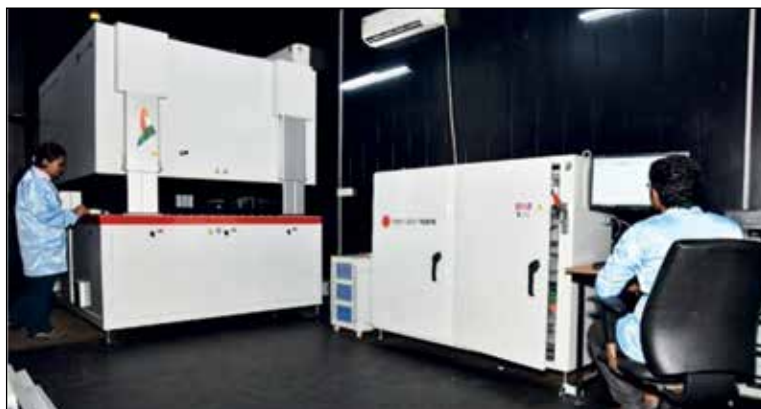
Fig. 10.1: Temperature Controlled Sun Simulator for testing of PV modules up to 650 W
