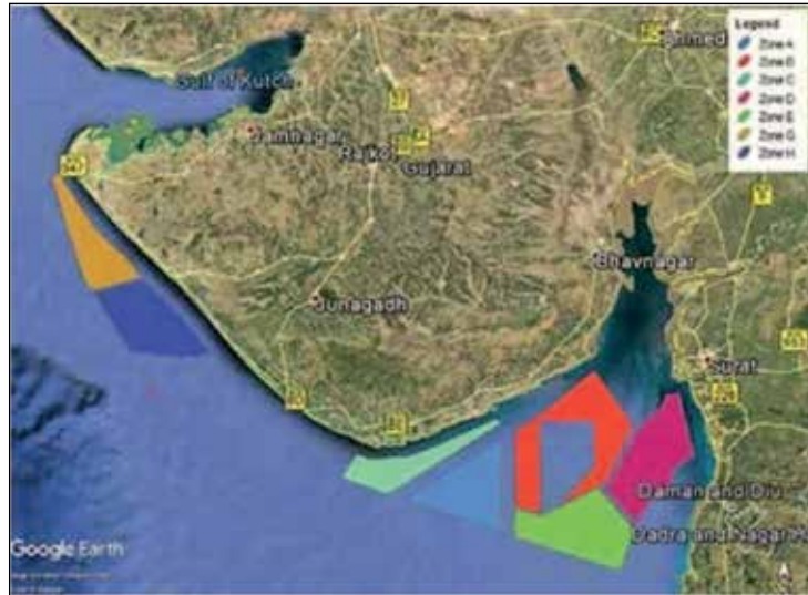
Fig. 4.2 Gujarat Offshore Wind Potential Zone
