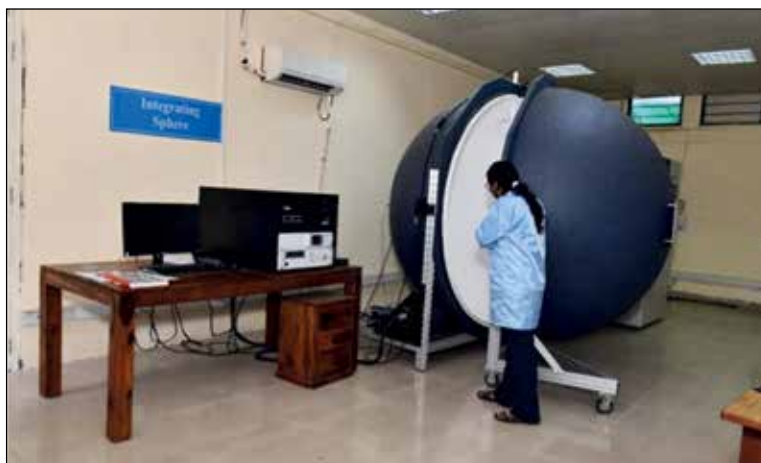
Fig.10.2: Testing of Solar Street Lights with Integrating sphere system
