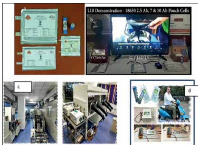
Fig. 7.4: (a) Prototype of 14 and 7 Ah NMC/graphite Li-ion pouch cells, Li-S pouch cell and 2.5-2.8 Ah NMC/graphite Li-ion cylindrical cells (b) Demonstration of the application of Li-ion pouch cells to operate a television, LED and table fan and its future application in isolated homes, (c) World class cell fabrication facility established at IIT Bombay, and (d) formed a start-up "Virya Batteries" with safe lithium ion battery and its demonstration.
