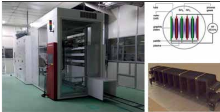
Fig. 7.12: PECVD installed at BHEL ASSCP (capable of processing depositing dielectric stack at rear side (AIOx with capping layer of SiONx/SiNx) and front side ARC)
