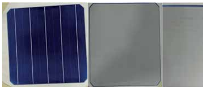
Fig. 7.2: Photographs of the front and backsides of the PERC cells fabricated at NCPRE
