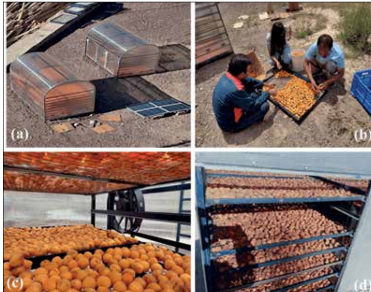
Fig. 10.5: Mini-Greenhouse based Solar Dryer: (a) Field testing in Ladakh, (b) Placing of apricots on mesh tray, (c) Fresh apricots fed inside the dryer, (d) Apricots during the drying process
