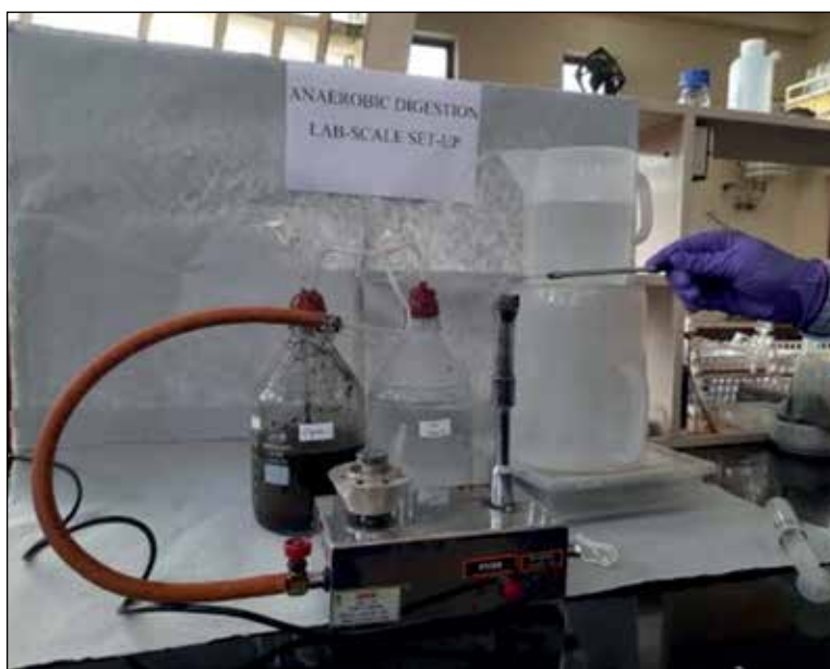
Fig. 10.17: Lab scale biogas plant using agricultural waste
