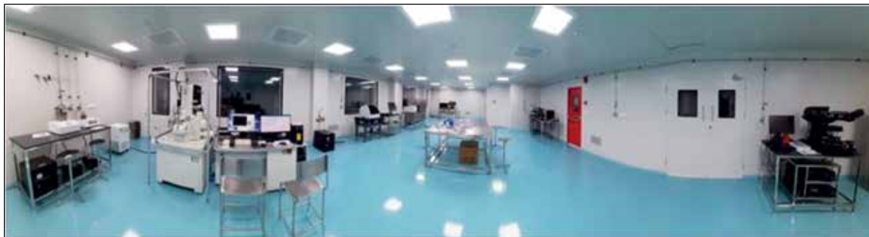
Fig. 10.3: Advanced Solar Cell characterization laboratory with ISO class 8 clean room facility at NISE
