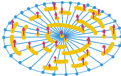
FIG. 3: Fragmented holographic geometry of an MBL system under the SBRG. Yellow blocks represent the Clifford gates, blue dots the physical qubits, and red arrows the emergent qubits. Adapted from [22].
