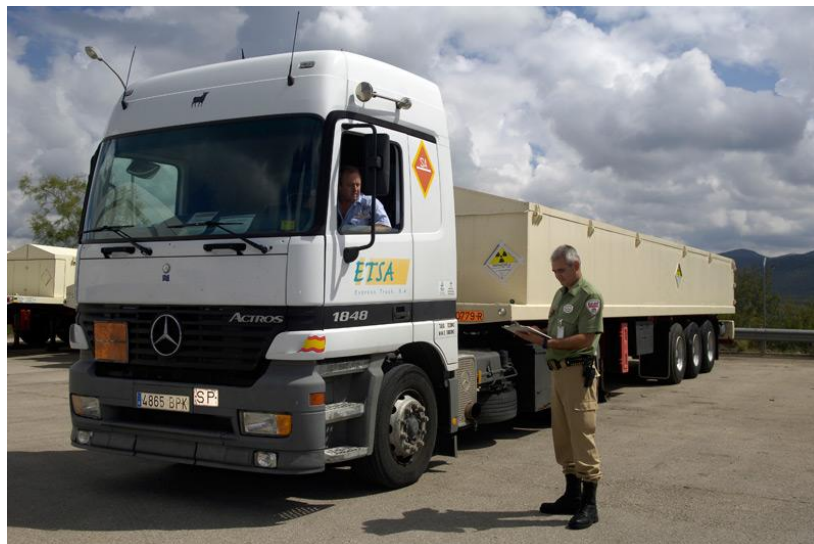
Figure 6. A truck used to transport LLW and ILW waste packages from different sites in Spain to El Cabril.
