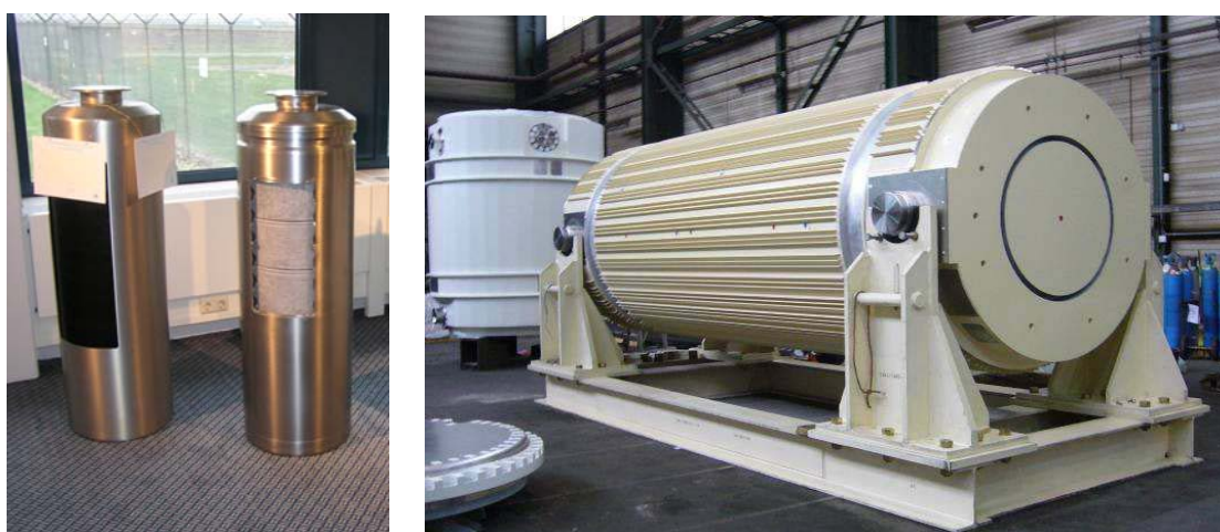
Figure 9. 500kg stainless steel canisters, used to store vitrified intermediate level waste from the reprocessing of ANSTO fuel (left) and the 100 tonne AREVA TN-81 transport and storage cask, capable of storing 28 canisters of ILW (right)
