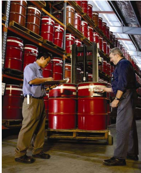
Figure 1. Storage of low level waste (LLW) at ANSTO. LLW contains low levels of radioactivity, and therefore shielding is not required to protect workers during storage or transportation.
