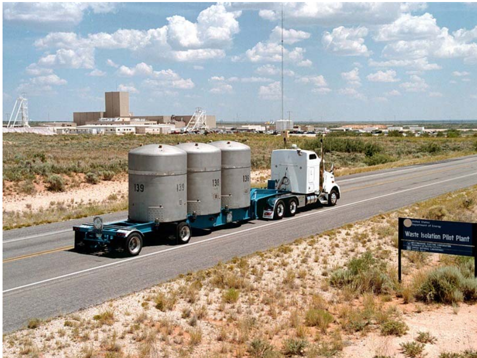
Figure 3. A truck transporting three casks of transuranic waste to the Waste Isolation Pilot Plant (WIPP) in New Mexico, USA
