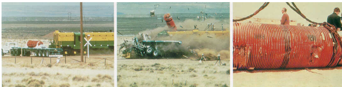
Figure 10. Impact testing of a transport cask conducted at US-DOE Sandia National Laboratory.
