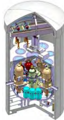
Figure 8: Schematics of varied DHR systems (normal and backup) and their integration in the guard containment vessel and containment building.
