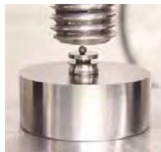
Figure 2: Equipment used at DOE/ORNL to measure strength of SiC and PyC.
