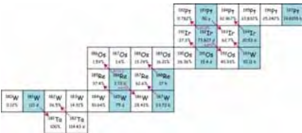
Figure 5: Transmutation cycle of Tungsten, Rhenium and Osmium, due to the neutronic captures; the blue boxes represent the unstable nuclei that decay through the purple arrows
