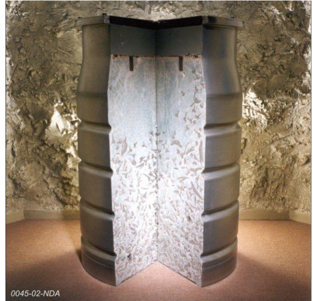
Cut-away showing intermediate level waste drum
