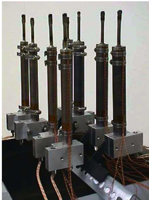
Figure 5.3-3. High-temperature water heat pipe testing.
