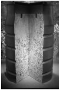
c) Long-lived intermediate-level waste from reprocessing spent Magnox fuel in 500-litre drum (courtesy of BNFL).
