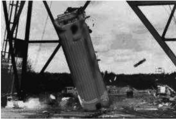
Fig. 5. Spent-fuel transportation cask undergoes a drop test (courtesy of GNS).
