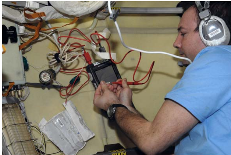
Figure 10-1. ISS018-E-027439 — Cosmonaut Yuri Lonchakov, Expedition 18 flight engineer, wears a hearing-protection device as he uses an oscilloscope to measure voltage in the Pirs docking compartment of the ISS (NASA Human Spaceflight Gallery, 2008).
