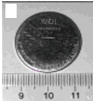
FIGURE 3: The optical image of an industry-grade coin-shaped graphene-based supercapacitor device. Reprinted with permission from Wang et al. [8] Copyright (2009) by American Chemical Society.
