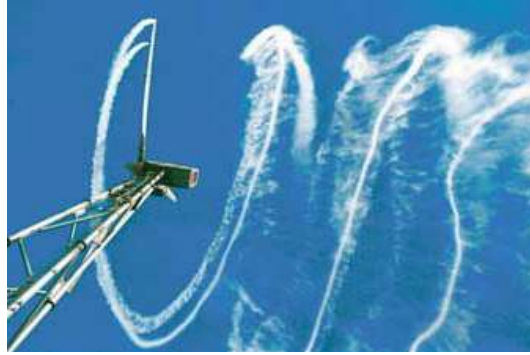
Figure 8 A demonstration of the wake formed behind a wind turbine using smoke. (Danish Wind Industry Association, 2003)
