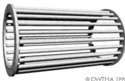
Figure 25 The cage part of ‘cage wound’ generator. (Danish Wind Industry Association, 2003)
