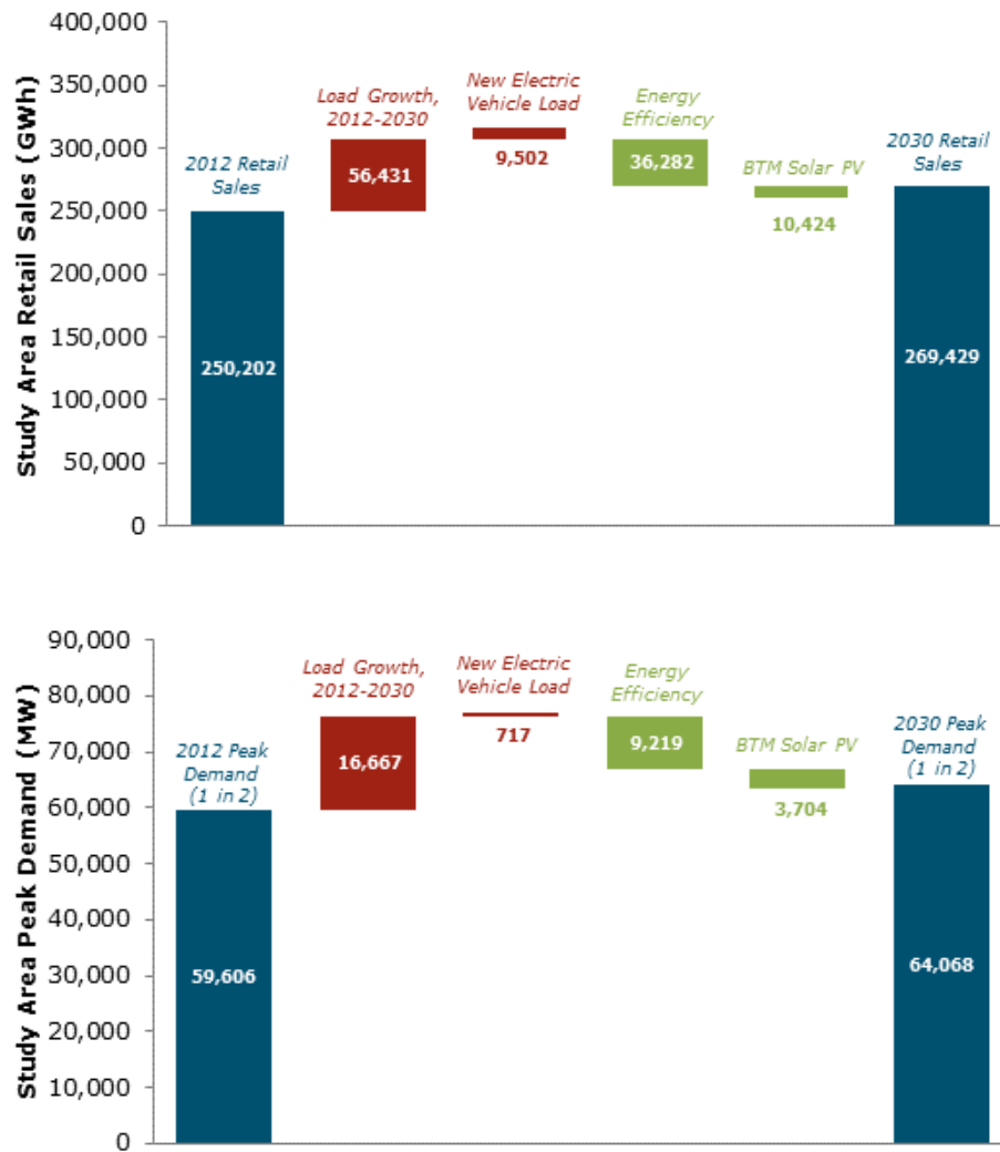
Figure 13: Changes to Study Area load, 2012 – 2030 for (top) retail sales and (bottom) peak demand
