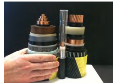
The 200 MW HVDC cable bundle is no more than 10 inches in diameter. The bundle shown in the picture is for transmission of 500 MW.
