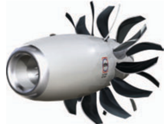
CFM International's open-rotor concept engine
