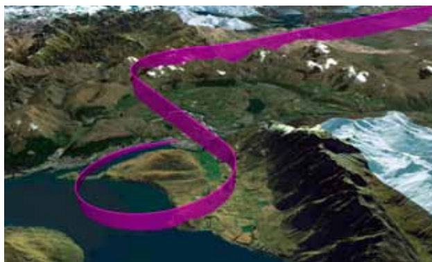
Required navigation performance procedures at Queenstown Airport in New Zealand have saved fuel and emissions for flights into this challenging airport.
