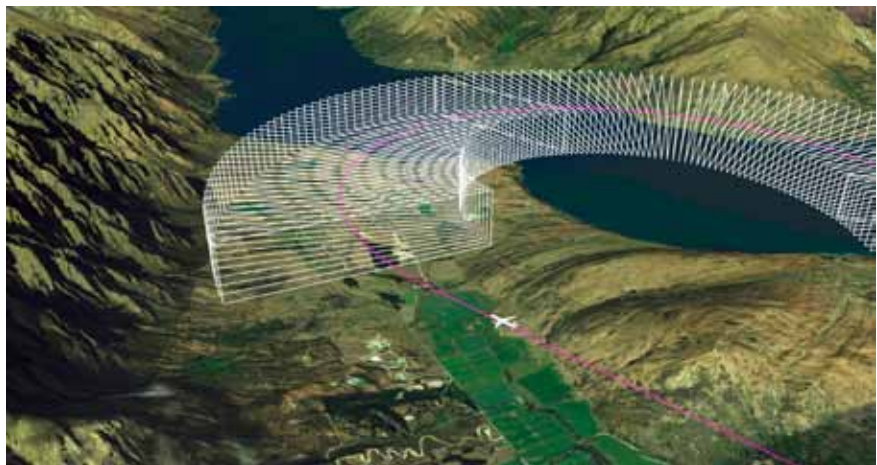
RNP technology defines a precise 'tunnel' through which an aircraft is programmed to fly.
