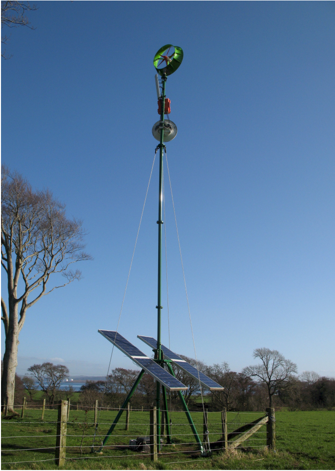
Fig. 2: Prototype “WindFi” base station on the Isle of Bute, Scotland, which has been running since early 2010. The base contains solar panels and batteries, over which a 10 m mast carries the wind turbine with antennas and radio equipment directly beneath.
