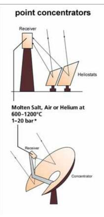
Figure 1 Technologies for concentrating solar radiation: left side parabolic and linear Fresnel troughs, right side central solar tower receiver and parabolic dish (Source: DLR)
