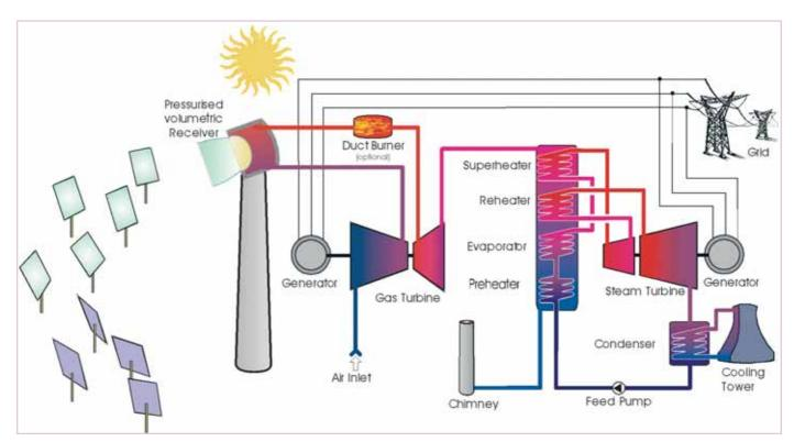
Schematic of a combined cycle system powered by a volumetric Figure 10 central receiver using pressurised air as heat transfer fluid (Source: DLR)
