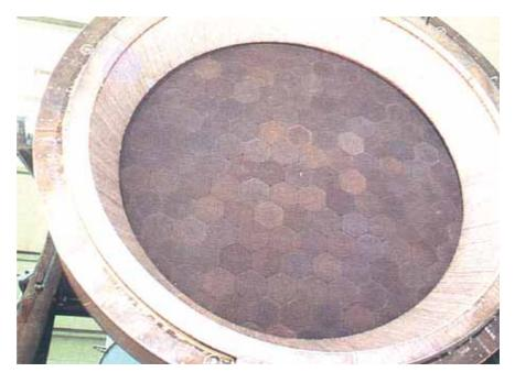
Figure 8 Volumetric receiver (Source: DLR)
