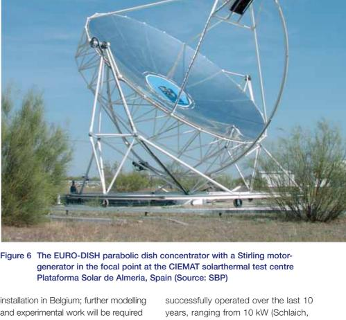
Figure 6 The EURO-DISH parabolic dish concentrator with a Stirling motor-
