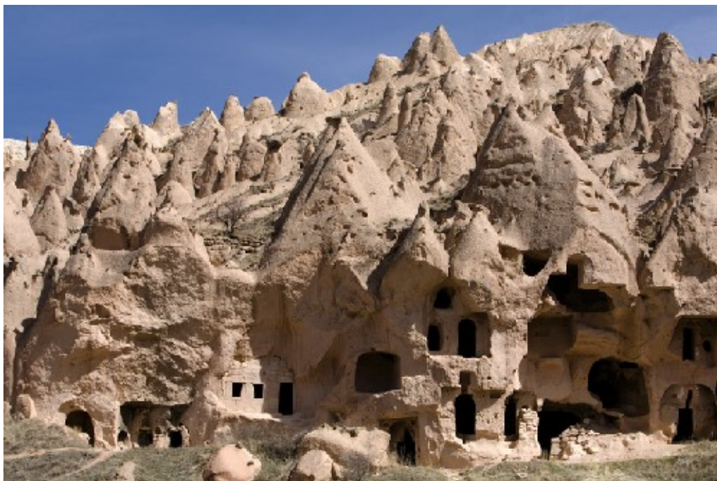
Fig.1. Occurring stable ground temperatures are utilized in Cappadocia (Turkey) where there are numerous buildings excavated in the mountains. The surrounding rock provides cooling in summer and heating in winter.
