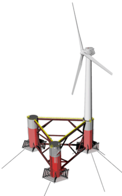
Figure 3: WindFloat semi-submersible modelled in TimeFloat [14]
